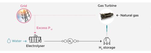
**Power to Hydrogen:** Development, integration and demonstration of power to hydrogen solution to increase the CC power plant flexibility and efficiency, while decreasing GHG emissions and use of natural gas.
