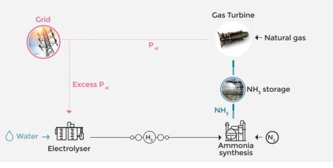
**Power to Ammonia:** Demonstration of power to ammonia solution at lab scale in a small-scale ammonia reactor for  $NH_3$ .
